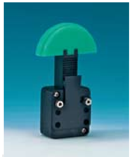
Spann-Box® designs with locking devices; they prevent the slide profile from being compressed when the direction of rotation changes, for example.
