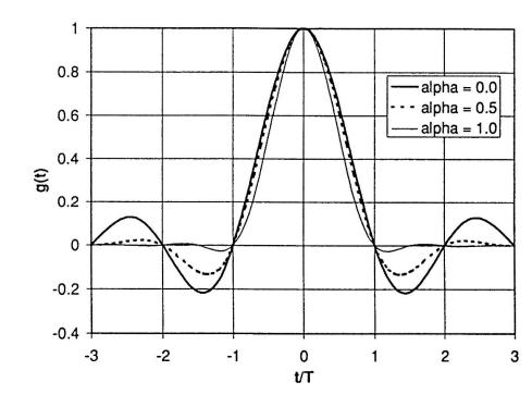
The roll-off factor, alpha, is a measure of the **excess bandwidth** of the filter, i.e. the **bandwidth** occupied beyond the Nyquist **bandwidth** of . ... This shows that the **excess bandwidth** of the filter can be reduced, but only at the expense of an elongated impulse response.
