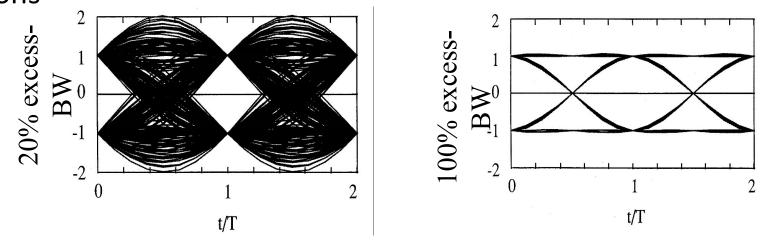
`eye diagram' is `oscilloscope view' of signal before sampler, when symbol timing serves as a trigger
